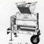
Shredder By W-W Grinder Corp.
