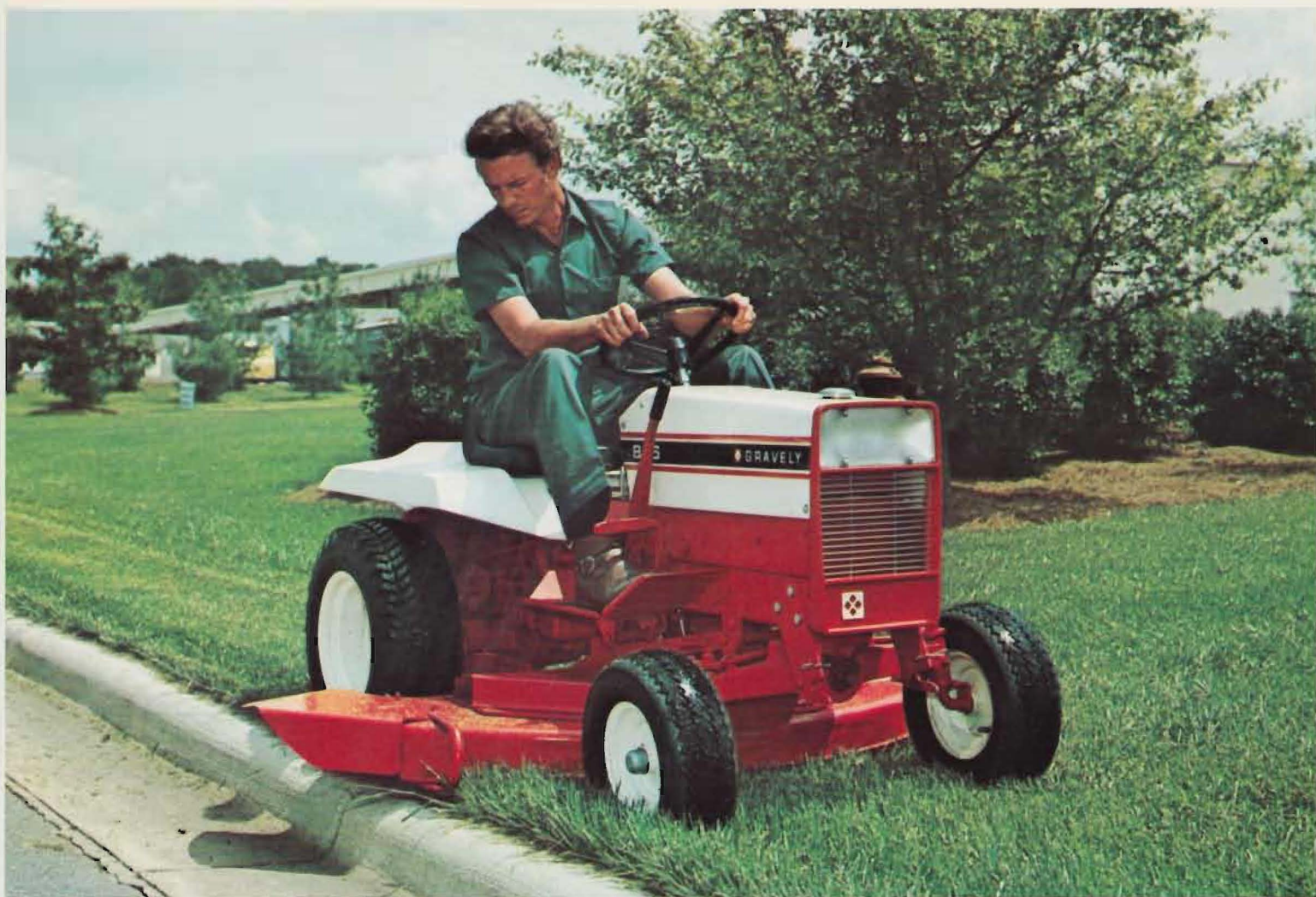
816, 16.5 HP Riding Tractor with 50-inch Center-Mount Rotary Mower.
