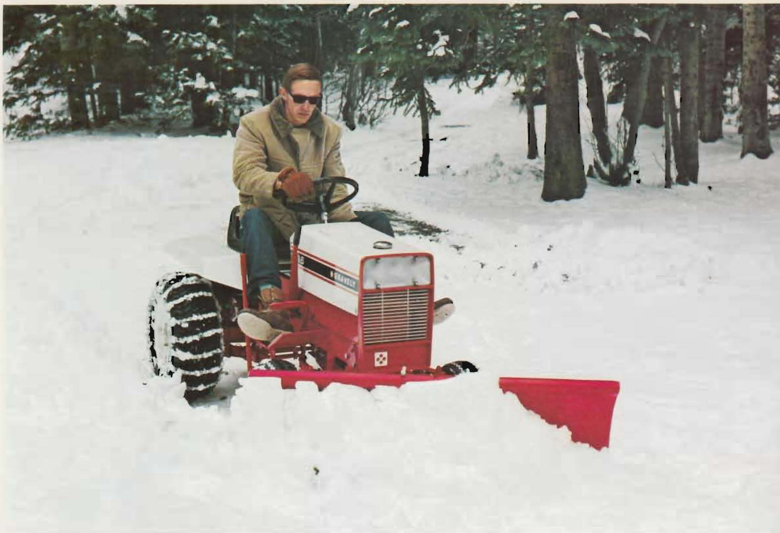
Gravely 816, 16.5 HP Riding Tractor with 48-inch SnowDozer, Optional Tire Chains and Wheel Weights.
