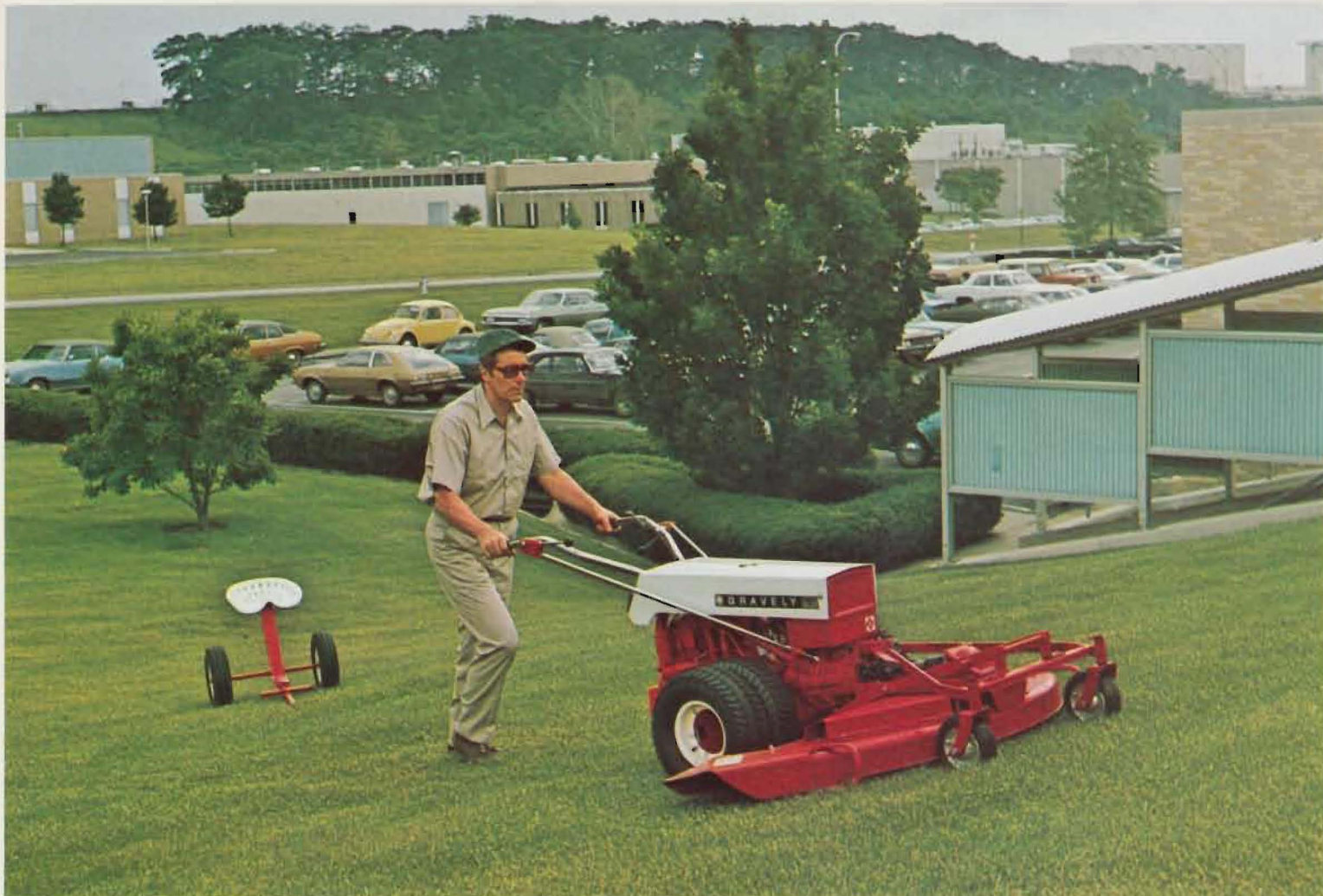
Gravely 12 HP Convertible Tractor with Quick Hitch Kit and 50-inch front mount Rotary Mower, Optional Dual Wheels, (Optional Riding Sulky in background)
