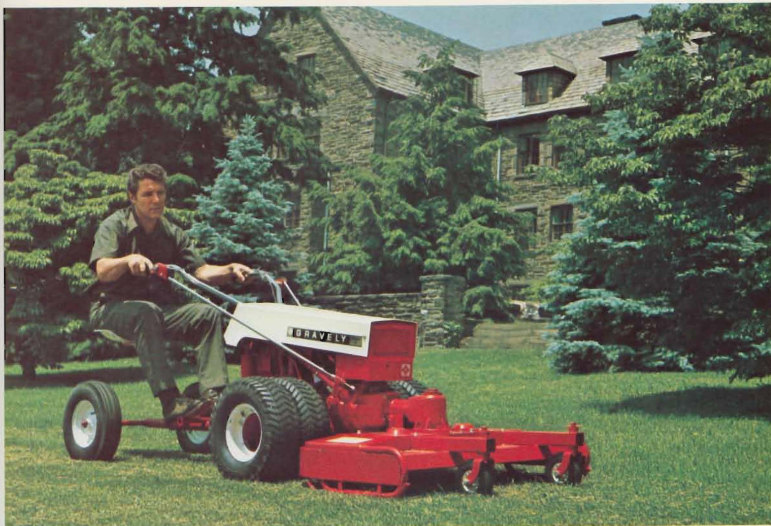
Gravely Commercial 12 Tractor with 40-inch Commercial Rotary Mower, Optional Dual Wheels, Riding Sulky and Trailing Hitch Kit.
