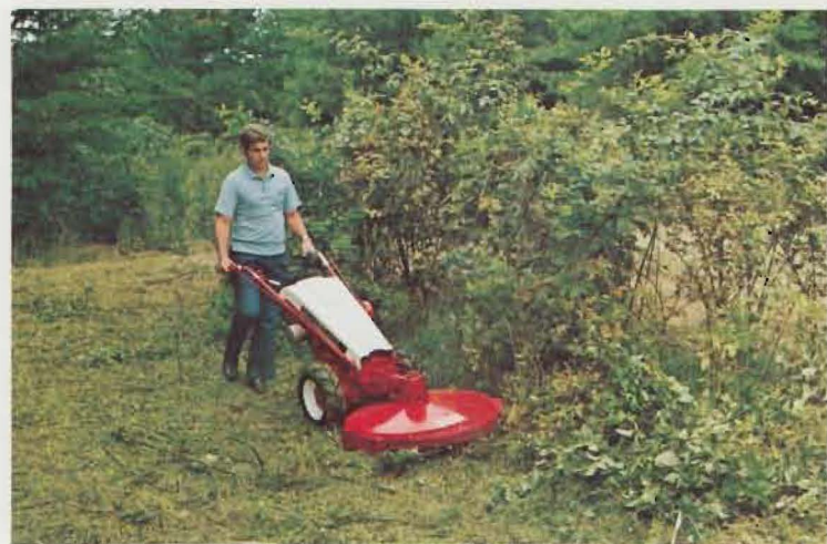
7.6 HP Custom Tractor (equipped with sure-grip tires) with 30-inch Rotary Mower-in the rough where power and all-gear-drive count.
