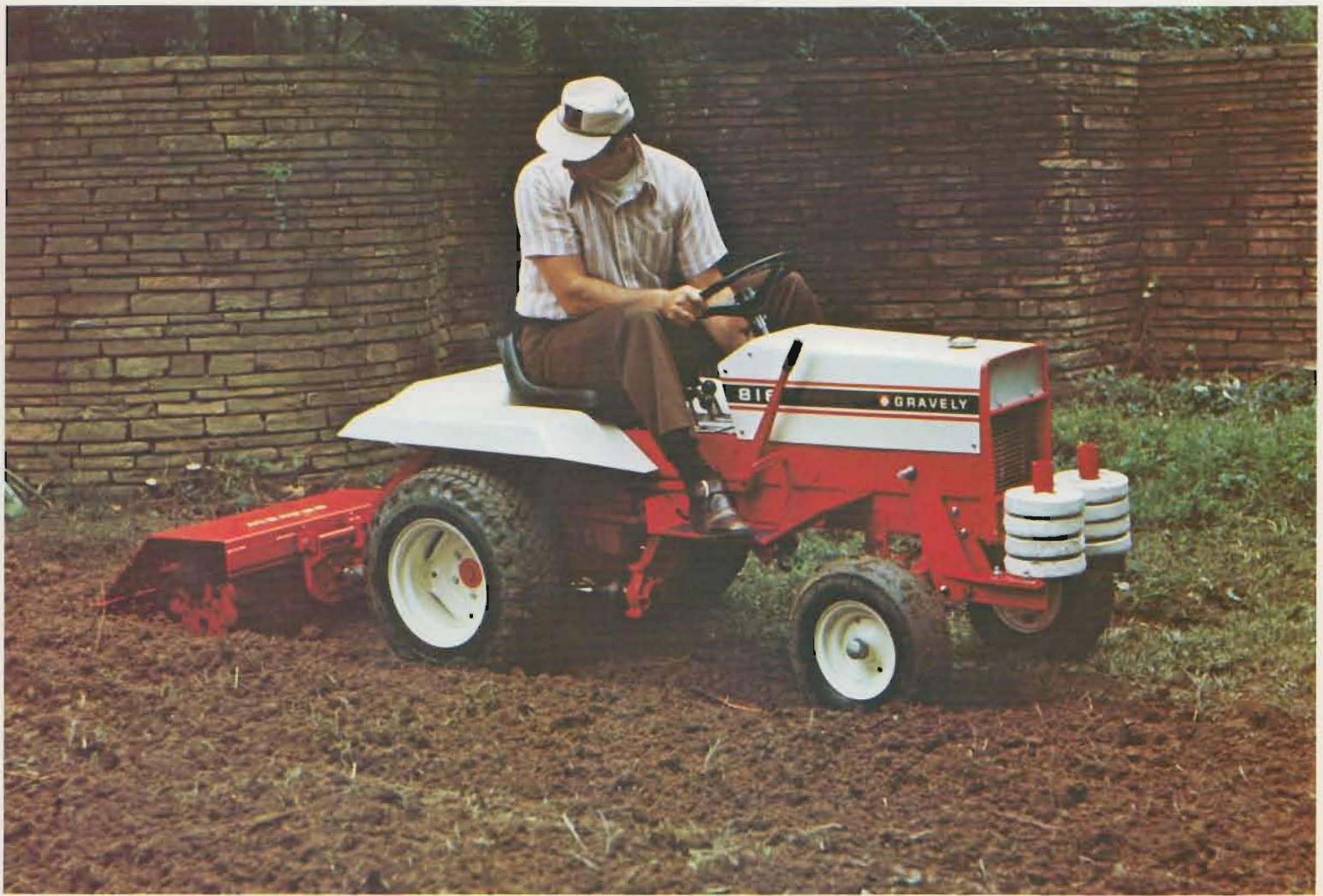
Gravely 816, 16.5 HP Riding Tractor with Rear Tiller, Optional Rear P.T.O. Kit, Optional Weight Rack Kit, plus weights.
