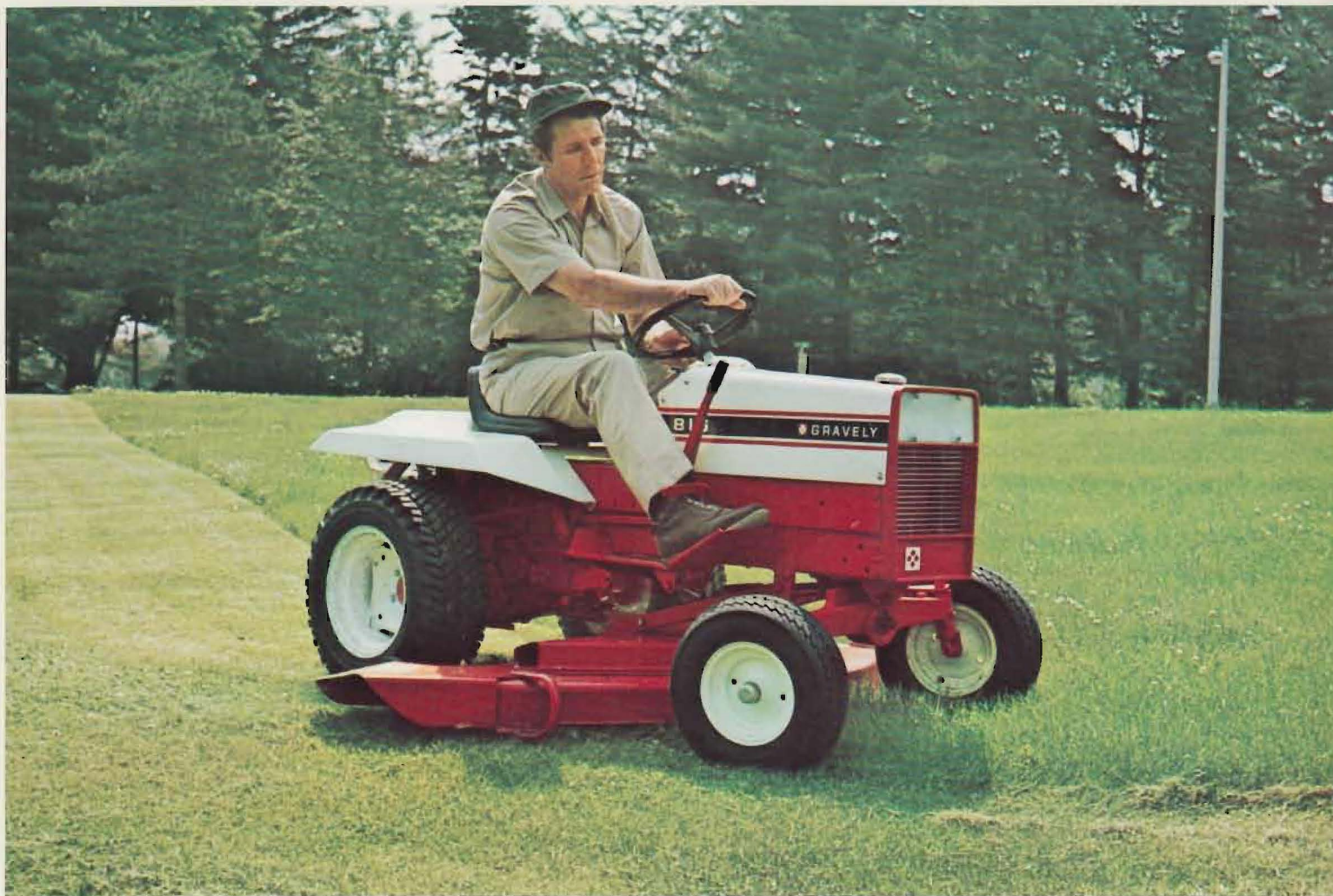
Gravely 816, 16.5 HP Riding Tractor with 50-inch Rotary Mower.
