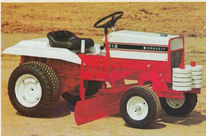
Gravely 812, 12 HP Riding Tractor with 48-inch Center-Mount Blade, Optional Front Weight Rack with Weights and Opt. Rear Wheel Weights.
