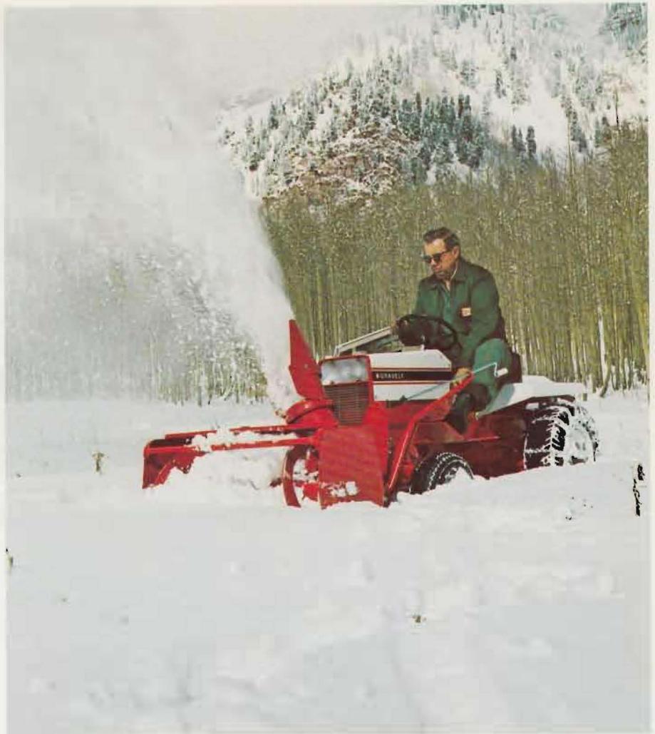
Gravelly 816S, 16 HP Riding Tractor with 38-inch Snowblower and Front Drive Kit, Optional factory-installed hydraulics, Optional Tire Chains and Wheel Weights.
